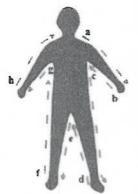
With the flat surface of the metal detector positioned parallel to the subject's torso, scan full area of the torso, down to the lower front portions of the subject; anatomy.
